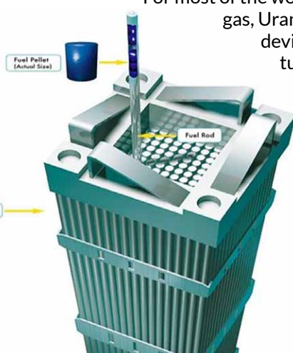
Illustration of a PWR fuel element of an array of 17x17 zircalloy tubes of 3.4m in length. Illustration shows Uranium oxide Fuel Pellets being loaded into the tubes.
